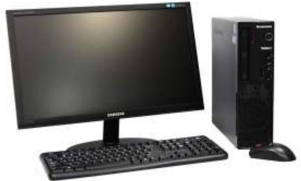
Core 2 Duo computer with TFT 22" screen Core 2 Duo con monitor TFT 22" (Lenovo Thinkcentre A70 Core2Duo 4Gb DDR3, D.D 500 GB)
