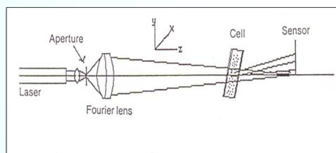
Figure 2. Light Scattering - Reverse Fourier Optics Technique.
