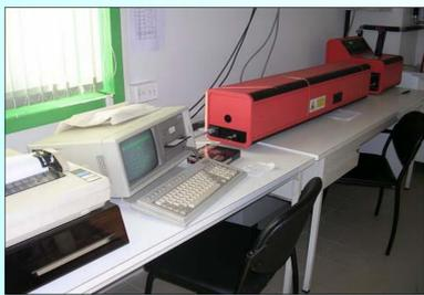
Figure 1. Helium - Neon Laser Particle Sizer Analysette 22, Fritsch & Gamble, D with interfaced computer for data processing.
