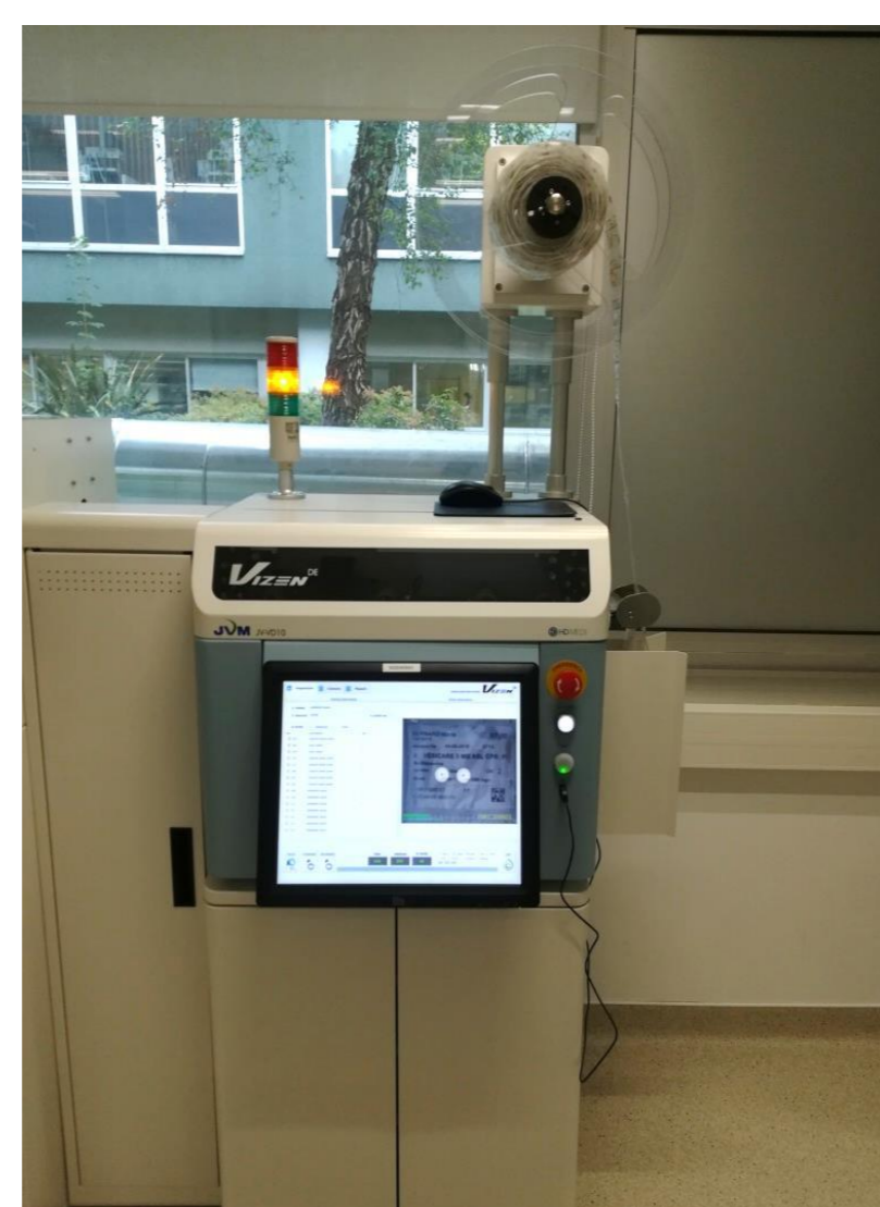
Automatic inspection machine : Vizen® (JVM®) takes photos of each unit dose and compares to its database
