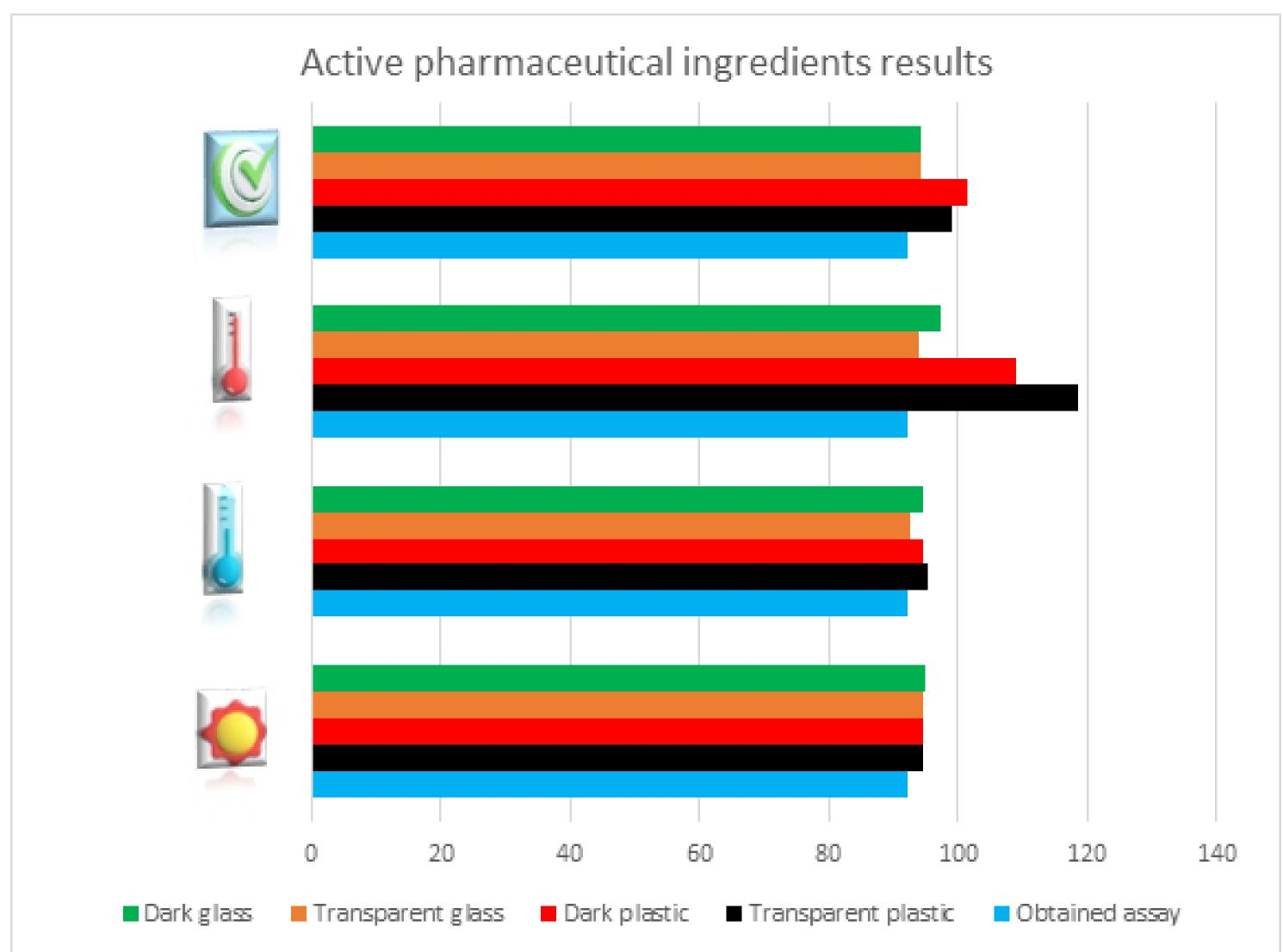
Solution was divided in glass (amber and transparent) and plastic (dark and transparent) bottles and stored at dark and cold place, elevated and decreased temperature.
