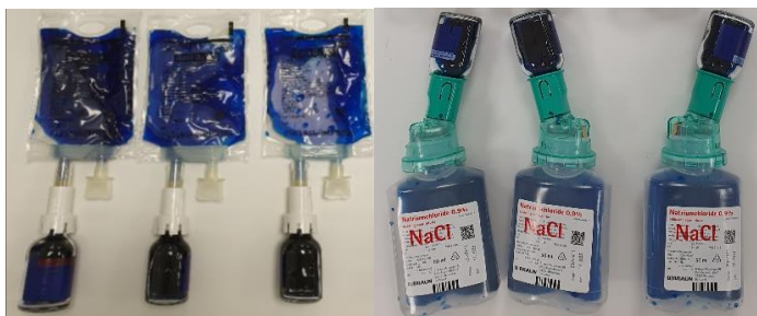
Figure 2. Three positive and negative controls of CSTD A (left) and B (right).
