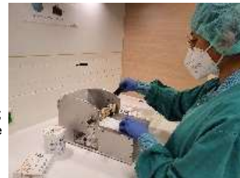
Fig.1: machine-aided deblistering of tablets; machine with bottom roll and adjustable discs operated with a manual crank
