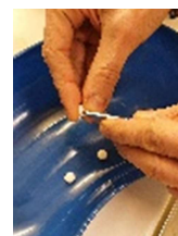
Fig.2: generation of tiny superficial defects on tablet film using a pointed item
