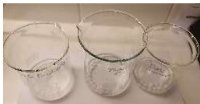
Fig.3: disintegration test TA in 0,1M HCl: minimally damaged (left), machine-deblistered (middle), manually deblistered (right)
